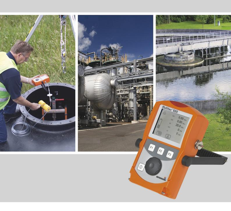
Versatile multiple gas warning device for workplace monitoring
