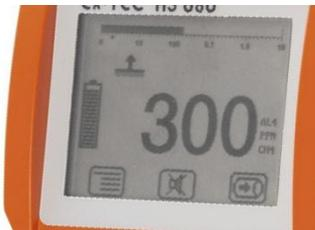
An important feature of the Variotec 460 tracer gas is that it contains 2 sensors. The low level sensor is used to measure very small levels of gas, parts per million (ppm), and the second sensor automatically measures the higher levels of gas, Vol %.
