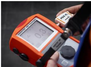
To check that the Variotec 460 is responding to hydrogen gas a key ring sized hydrogen generator is available. The PGG H2 generates a small quantity of hydrogen (ppm) . This is sampled by the VarioTec 460 which, if responding displays the indicated gas level on the large LCD.
