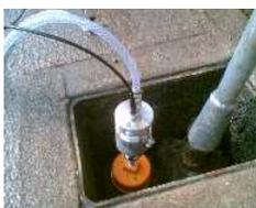
Standard piezo accelerometers listen to the leak noise on the surface of the pipe. Hydrophones are attached directly into the water column normally via hydrants. Leak noise can be heard far more successfully, over several hundred metres. They are particularly useful on plastic pipes and trunk mains where the leak noises frequency is likely to be lower than cast and steel pipes
