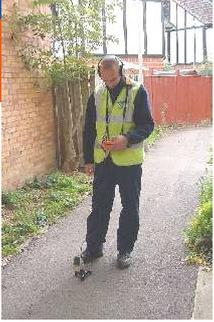
After correlation the indicated position should be checked by top sounding. With other correlators this means having to purchase a separate ground microphone - not so with the SeCorrPhon AC06. When used with the optional tripod foot the SeCorrPhon AC06 offers all the same functions as our Aquaphon ground microphone
